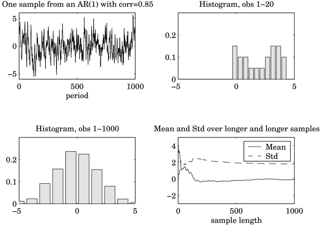
Figure 2.1: Sample of one realization of  $y_t = 0.85y_{t-1} + \varepsilon_t$  with  $y_0 = 4$  and  $\text{Std}(\varepsilon_t) = 1$ .
