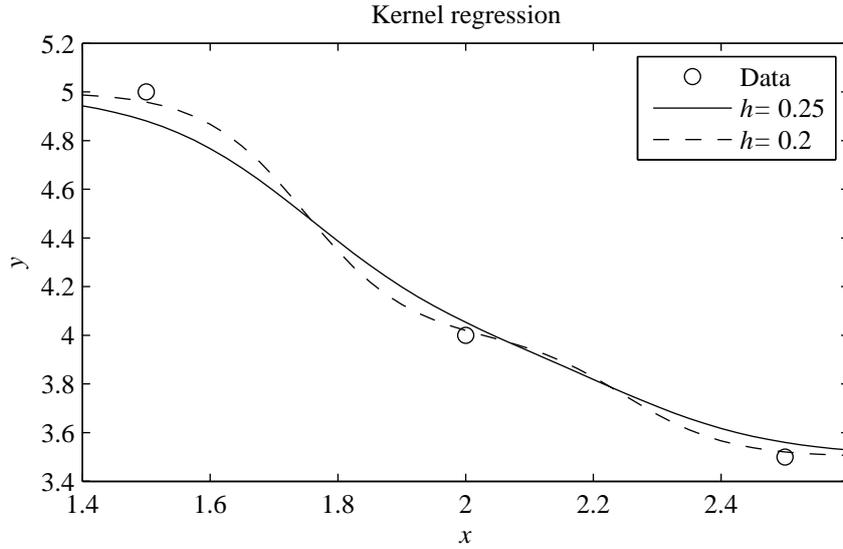
Figure 15.2: Example of kernel regression with three data points
