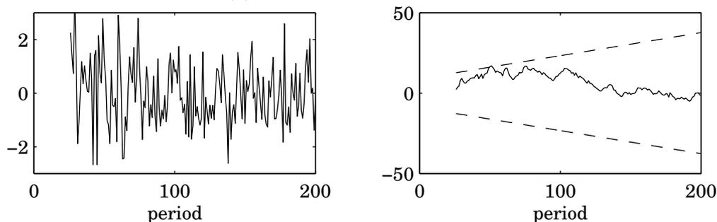
Figure 13.1: This figure shows recursive residuals and CUSUM statistics, when data are simulated from  $y_t = 0.85y_{t-1} + u_t$ , with  $\text{Var}(u_t) = 1$ .
