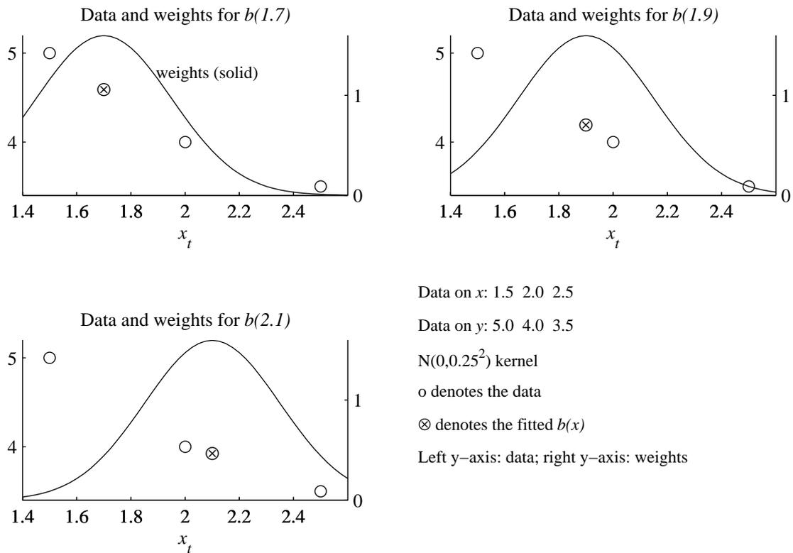
Figure 15.1: Example of kernel regression with three data points
