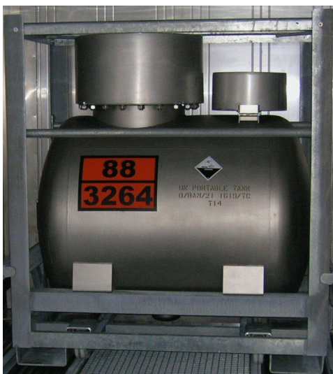
Fertiger Tankcontainer in Transportcontainer
